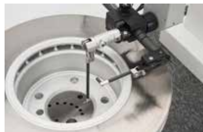
Special measuring station for specific tasks in brake disk measurement
