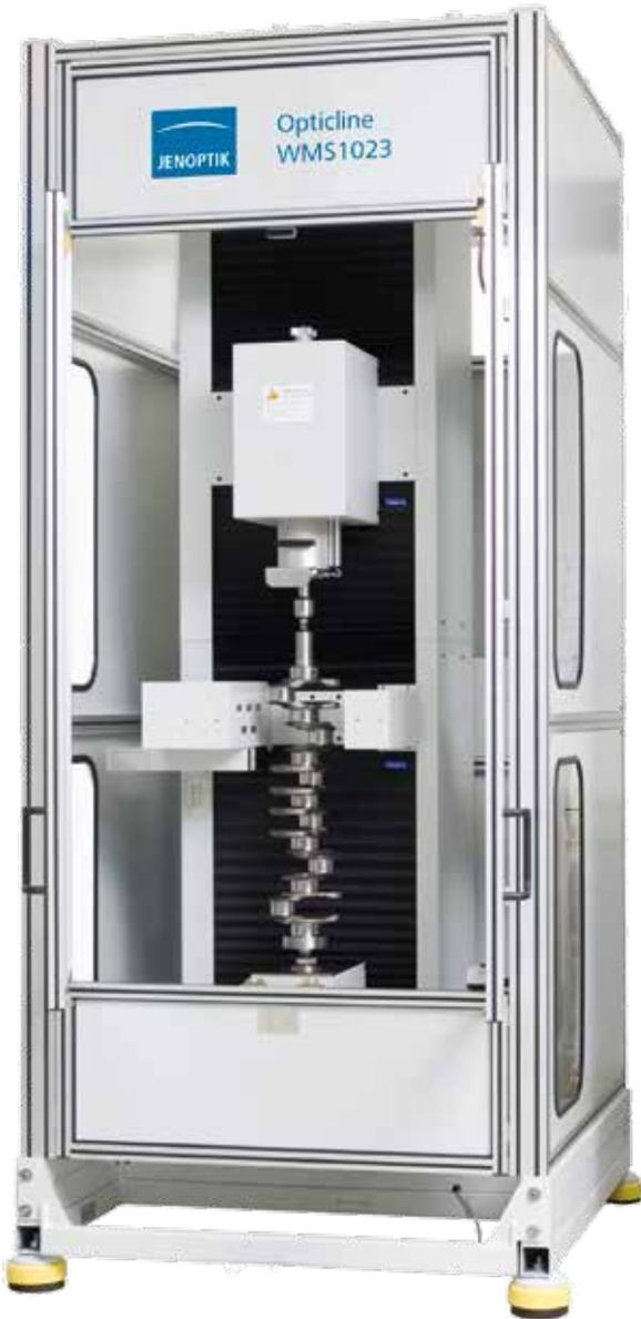
Opticline WMS1023 in a vertical design
