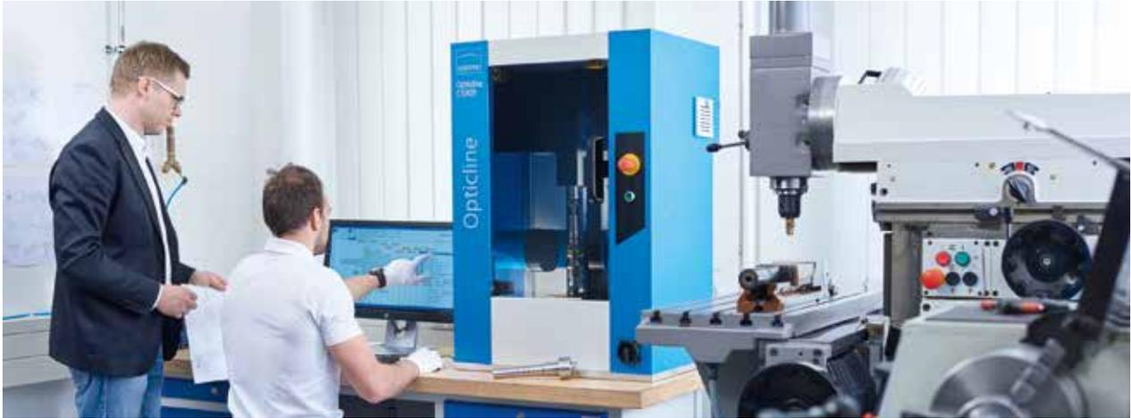
Opticline CS305 for cost-effective measurement of turned parts
