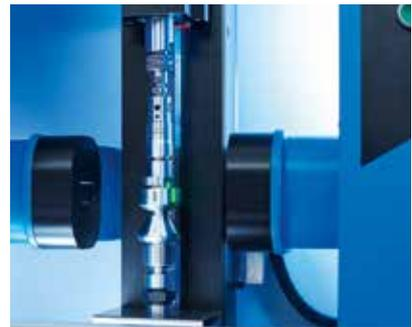
Simple clamping of the workpiece between tips
