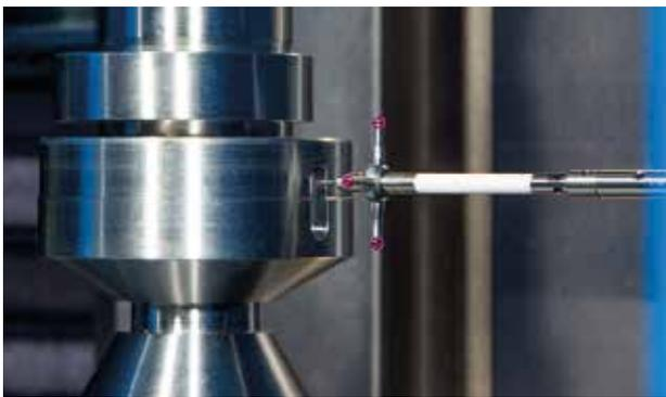
Probing system T3D for Opticline C series
