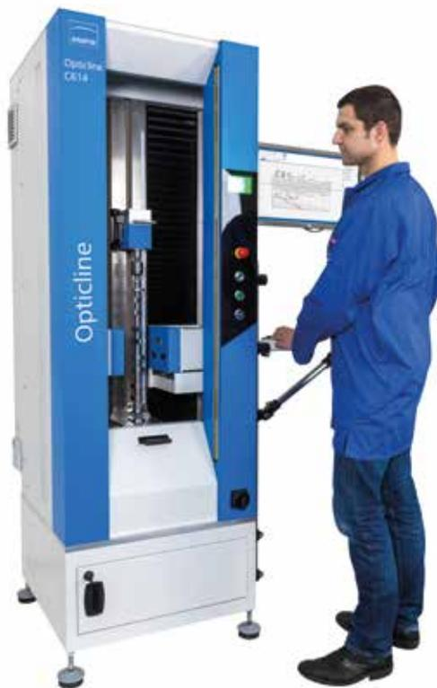
Our Opticline measuring solutions present a wide range of evaluation options and numerous areas of application for measuring shaft-type workpieces. Thanks to the fast, optical non-contact measuring principle, measurements are performed with an extremely high level of flexibility, repeatability and accuracy.
