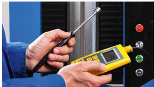
Workpiece temperature detection
