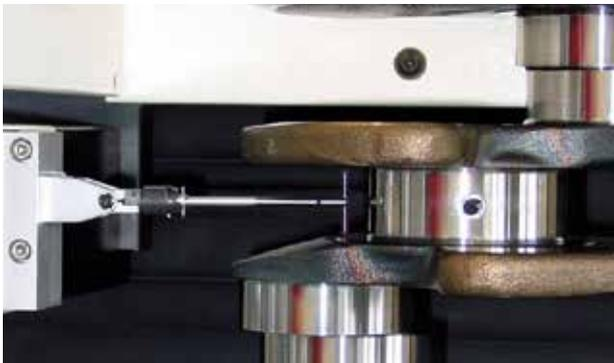
Probing system BTS for Opticline C1000, AMV and WMS
